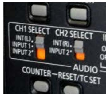
For each channel, the camera allows you to designate which source is recorded onto Channel 1 and Channel 2 of the audio tracks. INT (internal) for the microphone or EXT (external) for whatever is connected to the external connectors.
